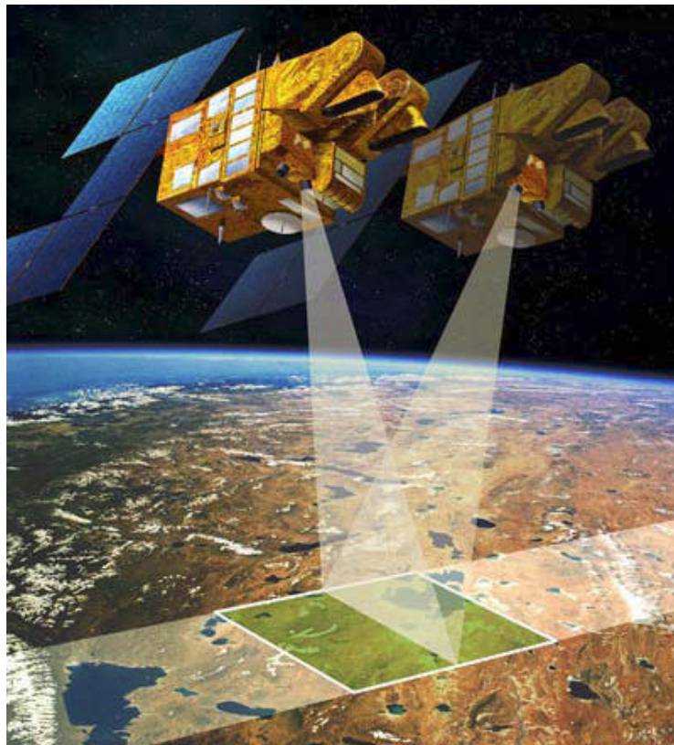
Figure 7: Stereo image acquisition by the SPOT 5 HRS instrument
